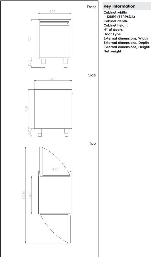
Modular Preparation 600 mm Passthrough Ambient Unit with 2 Doors
